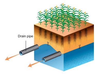
Figure 2. Diagram of a soil profile with subsurface (tile) drainage. Not to scale.
