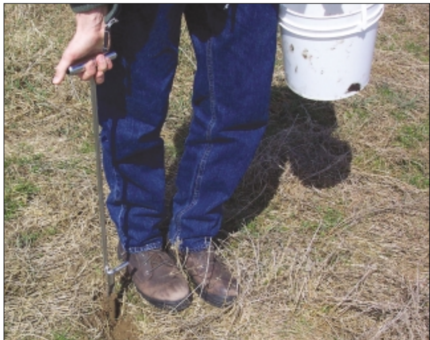
Collect soil cores with a sampling device like this step-in soil probe.
