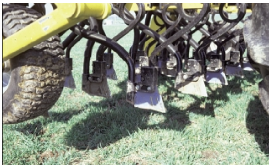
A no-till drill with coil tine and sod-slicing Baker Boot opener without a disc coulter used in overseeding pastures.
