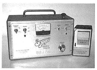
"Snoopy" – a device for measuring ethylene content of fruit under field conditons.
