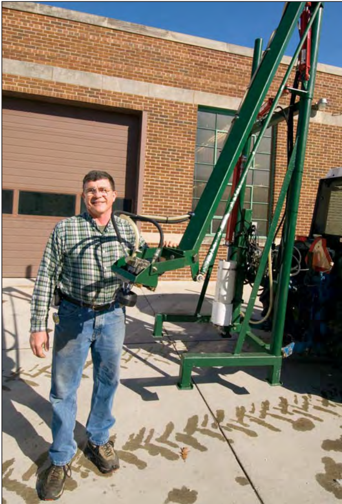
Richard Ledebuhr, former biosystems and agricultural engineering specialist, developed this spray mechanism to apply wax droplets to orchards. The wax is embedded with pheromone to control codling moth populations. MSU is now nationally known for its wax drop pheromone research.
