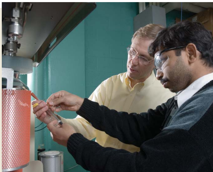
Dennis Miller (left) and Navin Asthana, postdoctoral associate, load a catalyst sample to analyze its metal content and surface area. Catalyst characterization is an important part of developing new technologies for value-added products from biomass.
