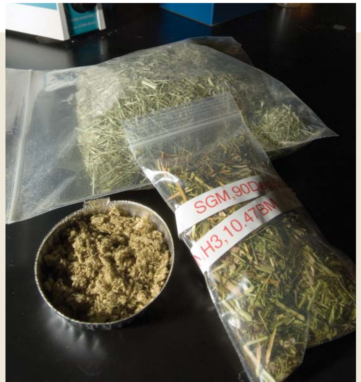
After biomass has been pretreated with Dale's AFEX process, more than 90 percent of the cellulose is broken down. When conventional methods are used, only about 15 percent of cellulose is broken down. Dale says that, after treatment, the plant material (at left) comes out somewhat like popcorn — slightly puffed up and dry.
