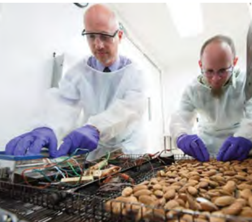
MAES scientist Brad Marks (left) and Mike James, lab manager of the biosafety level 2 pilot processing facility, attach sensors to almond samples for a food safety experiment.
